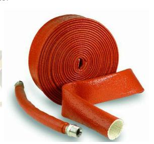
Pyrojacket features an excellent modulus of elasticity, allowing it to easily stretch and expand over fittings and connectors. The outer cover offers excellent resistance to most industrial chemicals and hydraulic oils. Additional uses include the bundling of multiple hoses and cables together, while providing good abrasion resistance.
